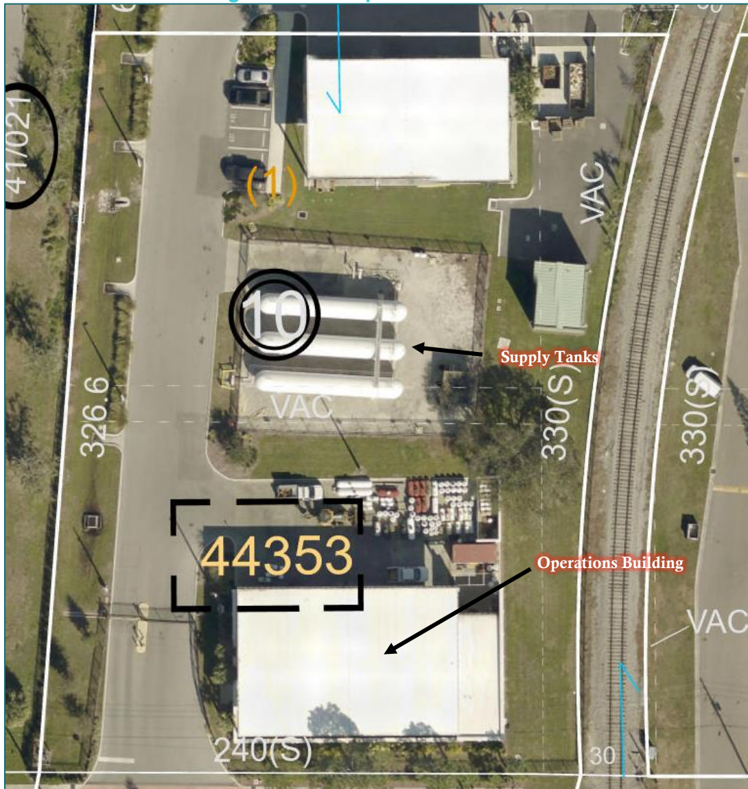
Figure 2-2: LP Operations Facilities
