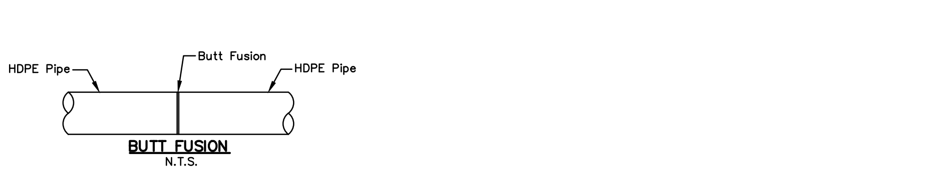
CITY OF CLEARWATER ENGINEERING DEPARTMENT RECLAIMED WATER DETAILS HDPE PIPE CONNECTIONS INDEX NO. 503 PAGE NO. 1 of 1 LATEST REVISION 7/2021
