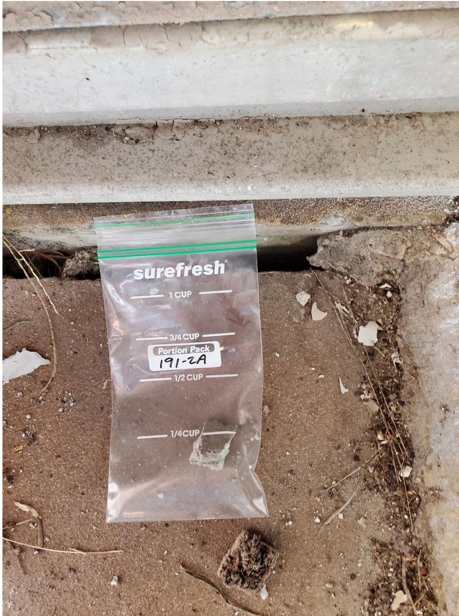
191-2A: Floor Caulk/Sealant [NAD]
